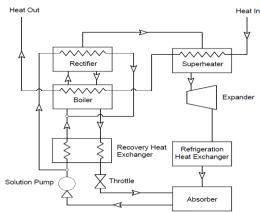
Fig: 6. Binary fluid (NH<sub>3</sub>-H<sub>2</sub>O) Thermal System [1]
