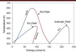
Fig: 4. Tempetrture-Entropy diagram of fluids [4]
