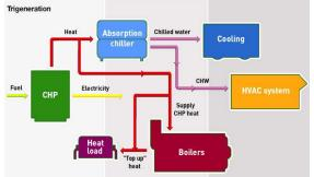
Fig: 2. Tri-generation System Layout [1]
