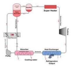
Fig: 7. Combined Rankine and Refrigeration cooling cycle-[1]
